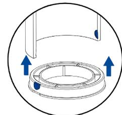
Schutzrohrglocke  $d = 100$  mm
